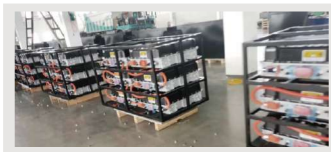
• 600V 350Ah battery system for mining truck
