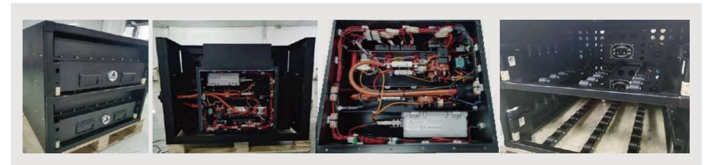
• 72V129Ah battery system for ATV
